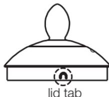
3. Adjust the tabs, replace the lid and remove it to see if the adjustment is correct.
